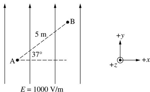
5. Points A and B are separated by a distance of 5 m and located in a uniform electric field of magnitude 1000 V/m directed in the  $+y$ -direction, as shown in the figure. The line between Point A and Point B makes an angle of  $37^\circ$  to the  $x$ -axis. When a proton (of charge  $+e$ ) is moved by an external force from Point A to Point B, what is the change in electric potential energy of the proton-field system?
