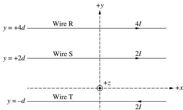
4. Three long wires, R, S, and T, are arranged in the  $xy$ -plane parallel to each other and the  $x$ -axis at the positions shown in the figure. The direction and current in each wire are indicated. Which of the following correctly indicates the magnitude and direction of the magnetic field at the origin of the coordinate system?
