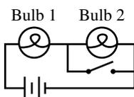
A circuit contains two identical lightbulbs and a switch connected to a battery, as shown. The switch is initially open.
