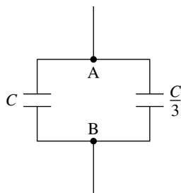
6. Two air-filled capacitors, with capacitance  $C$  and  $\frac{C}{3}$ , are connected in parallel, as shown. The equivalent capacitance between points A and B is  $C_{\text{eq}}$ . A dielectric is inserted into the capacitor with capacitance  $\frac{C}{3}$ , and the new equivalent capacitance between points A and B is  $2C_{\text{eq}}$ . What is the value of the dielectric constant of the dielectric?
