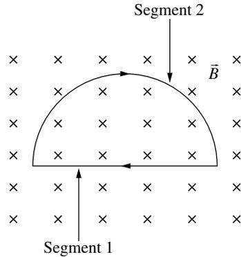
13. A semicircular loop with a clockwise current is placed in a uniform magnetic field that is directed into the page, as shown in the figure.  $\vec{F}_1$  is the net force on Segment 1, which is the straight portion of the loop.  $\vec{F}_2$  is the net force on Segment 2, which is the curved portion of the loop. Which of the following correctly indicates the directions and relative magnitudes of  $\vec{F}_1$  and  $\vec{F}_2$ ?
