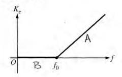
A is Planck's constant and B is the work function. fo is the threshold frequency at which electrons emit.
