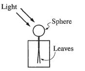
i. Ultraviolet (UV) light shines on the sphere, causing the leaves of the electroscope to move closer together. Explain why this happens.
