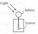
i. Ultraviolet (UV) light shines on the sphere, causing the leaves of the electroscope to move closer together. Explain why this happens.
