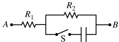
A second group of students is given a combination of circuit elements that is similar to the previous one but has an initially uncharged capacitor in series with the open switch, as shown above. The combination is placed in a circuit with a power supply so that the potential difference between A and B is maintained at 9 V. The students close the switch and immediately begin to record the current through point B. The initial current is 0.9 A, and after a long time the current is 0.3 A.
