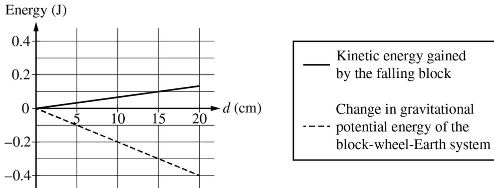
(c) The graph above represents both the change in the gravitational potential energy of the block-wheel-Earth system and the translational kinetic energy gained by the block as functions of the block’s falling distance  $d$ . On the graph, draw a line or curve to represent the rotational kinetic energy of the wheel as a function of the block’s falling distance  $d$ .
